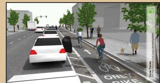
Cycle Track: Buffered, 6-11' wide.
