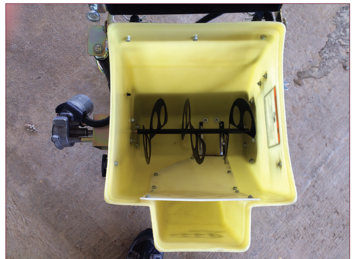
Figure 4. Specialized broadcast spreaders with agitators and picker wheels help spread light, fluffy seed mixes.
