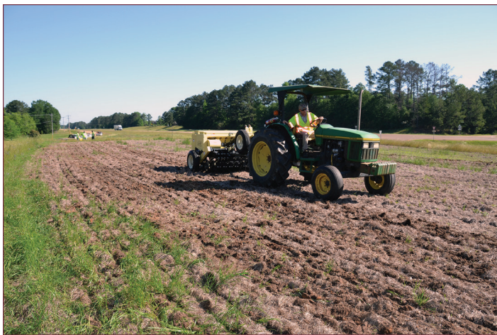
Figure 5. A no-till drill is useful in larger areas where tillage is not an option. Using a drill allows for less seed to be used because it is metered out, as opposed to being broadcast to the soil surface. Specialized drills allow for light, fluffy seed mixes to be easily planted.
